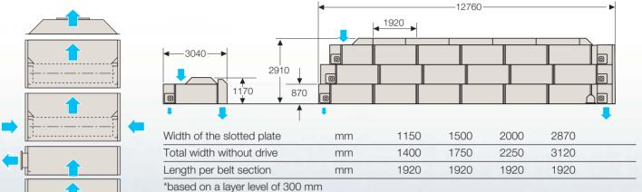
**Intermediate aspiration.** For the separation of the process sections, e.g. pre-cooling and post-cooling, pre-drying and post-drying, drying and cooling.
